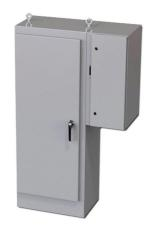
Saginaw enclosure, NEMA 3R/4/12/13, 72 x 28 x 18in (HxWxD), freestanding, carbon steel, ANSI 61 gray, powder coat finish, single-door, 3-point padlocking handle, external disconnect enclosure included.
