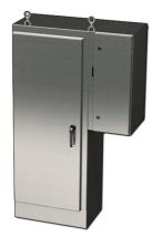
Saginaw enclosure, NEMA 3R/4/4X/12/13, 72 x 28 x 18in (HxWxD), freestanding, 304 stainless steel, #4 brush finish, single-door, 3-point padlocking handle, external disconnect enclosure included.
