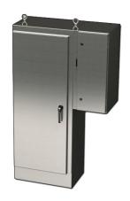
Saginaw enclosure, NEMA 3R/4/4X/12/13, 72 x 28 x 18in (HxWxD), freestanding, 316L stainless steel, #4 brush finish, single-door, 3-point padlocking handle, external disconnect enclosure included.
