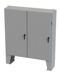
Saginaw disconnect enclosure, NEMA 3R/12/13, right flange,  $72 \times 73 \times 18$  in (HxWxD), floor mount, carbon steel, ANSI 61 gray, powder coat finish, 2-door, 3-point padlocking handle, purchase subpanel separately.
