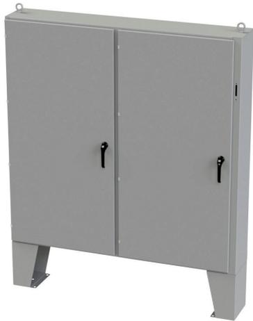
Saginaw disconnect enclosure, NEMA 3R/12/13, right flange, 72 x 73 x 12in (HxWxD), floor mount, carbon steel, ANSI 61 gray, powder coat finish, 2-door, 3-point padlocking handle, purchase subpanel separately.
