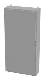
Saginaw enclosure, NEMA 3R/4/12/13, 72 x 36 x 12in (HxWxD), wall mount, carbon steel, ANSI 61 gray, powder coat finish, single-door, plated steel clamps, padlock hasp and staple.
