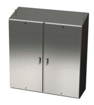
Saginaw Enviroline series enclosure, slope top, NEMA 3R/4/4X/12/13, 72 x 72 x 24in (HxWxD), freestanding, 304 stainless steel, #4 brush finish, 2-door, 3-point 304 stainless steel padlocking handle.
