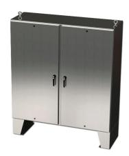
Saginaw Enviroline series enclosure, NEMA 3R/4/4X/12/13, 72 x 72 x 24in (HxWxD), floor mount, 304 stainless steel, #4 brush finish, 2-door, 3-point keylocking/padlocking combo handle.
