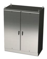
Saginaw Enviroline series enclosure, NEMA 3R/4/4X/12/13, 72 x 72 x 24in (HxWxD), freestanding, 304 stainless steel, #4 brush finish, 2-door, 3-point keylocking/padlocking combo handle.
