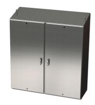
Saginaw Enviroline series enclosure, slope top, NEMA 3R/4/4X/12/13, 72 x 72 x 24in (HxWxD), freestanding, 316L stainless steel, #4 brush finish, 2-door, 3-point 304 stainless steel padlocking handle.
