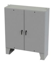
Saginaw Enviroline series enclosure, NEMA 3R/4/12/13, 72 x 72 x 24in (HxWxD), floor mount, carbon steel, ANSI 61 gray, powder coat finish, 2-door, 3-point keylocking/padlocking combo handle.
