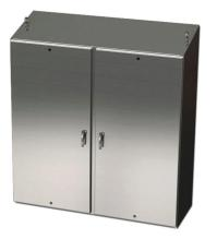
Saginaw Enviroline series enclosure, slope top, NEMA 3R/4/4X/12/13, 72 x 72 x 18in (HxWxD), freestanding, 304 stainless steel, #4 brush finish, 2-door, 3-point 304 stainless steel padlocking handle.
