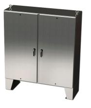
Saginaw Enviroline series enclosure, NEMA 3R/4/4X/12/13, 72 x 72 x 18in (HxWxD), floor mount, 304 stainless steel, #4 brush finish, 2-door, 3-point keylocking/padlocking combo handle.
