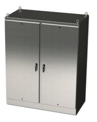
Saginaw Enviroline series enclosure, NEMA 3R/4/4X/12/13, 72 x 72 x 18in (HxWxD), freestanding, 304 stainless steel, #4 brush finish, 2-door, 3-point keylocking/padlocking combo handle.
