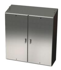
Saginaw Enviroline series enclosure, slope top, NEMA 3R/4/4X/12/13, 72 x 72 x 18in (HxWxD), freestanding, 316L stainless steel, #4 brush finish, 2-door, 3-point 304 stainless steel padlocking handle.
