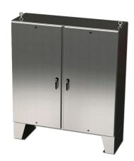
Saginaw Enviroline series enclosure, NEMA 3R/4/4X/12/13, 72 x 72 x 18in (HxWxD), floor mount, 316L stainless steel, #4 brush finish, 2-door, 3-point keylocking/padlocking combo handle.
