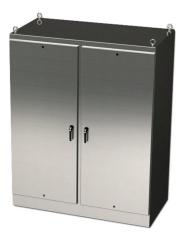
Saginaw Enviroline series enclosure, NEMA 3R/4/4X/12/13, 72 x 72 x 18in (HxWxD), freestanding, 316L stainless steel, #4 brush finish, 2-door, 3-point keylocking/padlocking combo handle.
