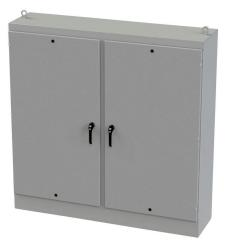
Saginaw Enviroline series enclosure, NEMA 3R/4/12/13, 72 x 72 x 18in (HxWxD), freestanding, carbon steel, ANSI 61 gray, powder coat finish, 2-door, 3-point keylocking/padlocking combo handle.
