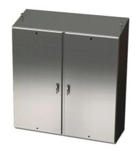
Saginaw Enviroline series enclosure, slope top, NEMA 3R/4/4X/12/13, 72 x 72 x 12in (HxWxD), freestanding, 304 stainless steel, #4 brush finish, 2-door, 3-point 304 stainless steel padlocking handle.
