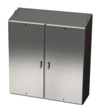
Saginaw Enviroline series enclosure, slope top, NEMA 3R/4/4X/12/13,  $72 \times 72 \times 12$  in (HxWxD), freestanding, 316L stainless steel, #4 brush finish, 2-door, 3-point 304 stainless steel padlocking handle.
