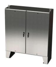
Saginaw Enviroline series enclosure, NEMA 3R/4/4X/12/13, 72 x 72 x 12in (HxWxD), floor mount, 316L stainless steel, #4 brush finish, 2-door, 3-point keylocking/padlocking combo handle.
