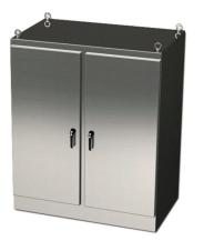
Saginaw Enviroline series enclosure, NEMA 3R/4/4X/12/13, 72 x 60 x 36in (HxWxD), freestanding, 304 stainless steel, #4 brush finish, 2-door, 3-point keylocking/padlocking combo handle.
