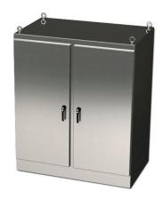
Saginaw Enviroline series enclosure, NEMA 3R/4/4X/12/13, 72 x 60 x 36in (HxWxD), freestanding, 316L stainless steel, #4 brush finish, 2-door, 3-point keylocking/padlocking combo handle.
