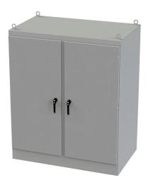
Saginaw Enviroline series enclosure, NEMA 3R/4/12/13, 72 x 60 x 36in (HxWxD), freestanding, carbon steel, ANSI 61 gray, powder coat finish, 2-door, 3-point keylocking/padlocking combo handle.
