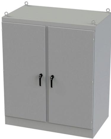
Saginaw Enviroline series enclosure, NEMA 3R/4/12/13, 72 x 60 x 36in (HxWxD), freestanding, carbon steel, ANSI 61 gray, powder coat finish, 2-door, 3-point keylocking/padlocking combo handle.
