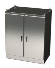
Saginaw Enviroline series enclosure, NEMA 3R/4/4X/12/13, 72 x 60 x 24in (HxWxD), freestanding, 304 stainless steel, #4 brush finish, 2-door, 3-point keylocking/padlocking combo handle.
