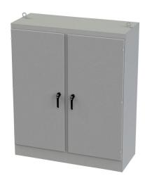
Saginaw Enviroline series enclosure, NEMA 3R/4/12/13, 72 x 60 x 24in (HxWxD), freestanding, carbon steel, ANSI 61 gray, powder coat finish, 2-door, 3-point keylocking/padlocking combo handle.
