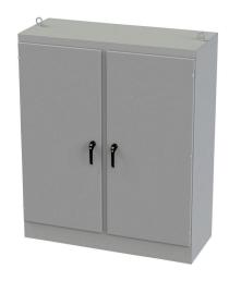
Saginaw Enviroline series enclosure, NEMA 3R/4/12/13, 72 x 60 x 24in (HxWxD), freestanding, carbon steel, ANSI 61 gray, powder coat finish, 2-door, 3-point keylocking/padlocking combo handle.
