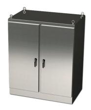
Saginaw Enviroline series enclosure, NEMA 3R/4/4X/12/13,  $72 \times 60 \times 18$ in (HxWxD), freestanding, 304 stainless steel, #4 brush finish, 2-door, 3-point keylocking/padlocking combo handle.
