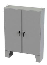
Saginaw Enviroline series enclosure, NEMA 3R/4/12/13, 72 x 60 x 18in (HxWxD), floor mount, carbon steel, ANSI 61 gray, powder coat finish, 2-door, 3-point keylocking/padlocking combo handle.
