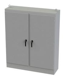
Saginaw Enviroline series enclosure, NEMA 3R/4/12/13,  $72 \times 60 \times 18$  in (HxWxD), freestanding, carbon steel, ANSI 61 gray, powder coat finish, 2-door, 3-point keylocking/padlocking combo handle.
