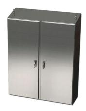
Saginaw Enviroline series enclosure, slope top, NEMA 3R/4/4X/12/13, 72 x 60 x 12in (HxWxD), freestanding, 304 stainless steel, #4 brush finish, 2-door, 3-point 304 stainless steel padlocking handle.
