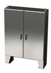
Saginaw Enviroline series enclosure, NEMA 3R/4/4X/12/13, 72 x 60 x 12in (HxWxD), floor mount, 304 stainless steel, #4 brush finish, 2-door, 3-point keylocking/padlocking combo handle.
