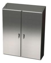
Saginaw Enviroline series enclosure, slope top, NEMA 3R/4/4X/12/13, 72 x 60 x 12in (HxWxD), freestanding, 316L stainless steel, #4 brush finish, 2-door, 3-point 304 stainless steel padlocking handle.
