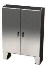
Saginaw Enviroline series enclosure, NEMA 3R/4/4X/12/13, 72 x 60 x 12in (HxWxD), floor mount, 316L stainless steel, #4 brush finish, 2-door, 3-point keylocking/padlocking combo handle.
