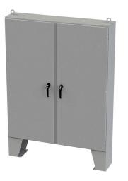
Saginaw Enviroline series enclosure, NEMA 3R/4/12/13, 72 x 60 x 12in (HxWxD), floor mount, carbon steel, ANSI 61 gray, powder coat finish, 2-door, 3-point keylocking/padlocking combo handle.
