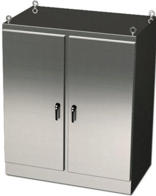
Saginaw Enviroline series enclosure, NEMA 3R/4/4X/12/13, 72 x 48 x 24in (HxWxD), freestanding, 304 stainless steel, #4 brush finish, 2-door, 3-point keylocking/padlocking combo handle.
