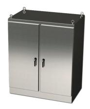
Saginaw Enviroline series enclosure, NEMA 3R/4/4X/12/13, 72 x 48 x 24in (HxWxD), freestanding, 316L stainless steel, #4 brush finish, 2-door, 3-point keylocking/padlocking combo handle.
