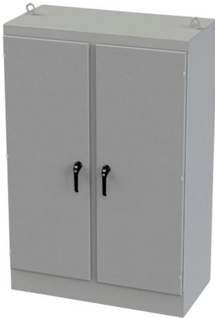
Saginaw Enviroline series enclosure, NEMA 3R/4/12/13, 72 x 48 x 24in (HxWxD), freestanding, carbon steel, ANSI 61 gray, powder coat finish, 2-door, 3-point keylocking/padlocking combo handle.
