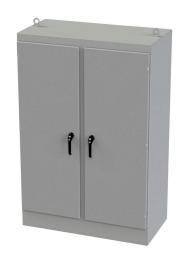
Saginaw Enviroline series enclosure, NEMA 3R/4/12/13, 72 x 48 x 24in (HxWxD), freestanding, carbon steel, ANSI 61 gray, powder coat finish, 2-door, 3-point keylocking/padlocking combo handle.
