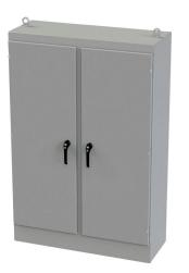
Saginaw Enviroline series enclosure, NEMA 3R/4/12/13, 72 x 48 x 18in (HxWxD), freestanding, carbon steel, ANSI 61 gray, powder coat finish, 2-door, 3-point keylocking/padlocking combo handle.
