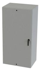
Saginaw Enviroline series enclosure, NEMA 3R/4/12/13, 72 x 36 x 24in (HxWxD), wall mount, carbon steel, ANSI 61 gray, powder coat finish, single-door, 3-point keylocking/padlocking combo handle.
