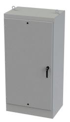
Saginaw Enviroline series enclosure, NEMA 3R/4/12/13, 72 x 36 x 24in (HxWxD), freestanding, carbon steel, ANSI 61 gray, powder coat finish, single-door, 3-point keylocking/padlocking combo handle.
