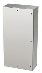
Saginaw Enviroline series enclosure, NEMA 3R/4/4X/12/13, 72 x 36 x 16in (HxWxD), wall mount, 304 stainless steel, #4 brush finish, single-door, 1/4-turn semi-flush latch.
