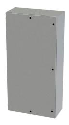
Saginaw Enviroline series enclosure, NEMA 3R/4/12/13, 72 x 36 x 16in (HxWxD), wall mount, carbon steel, ANSI 61 gray, powder coat finish, single-door, 1/4-turn semi-flush latch.
