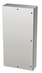
Saginaw Enviroline series enclosure, NEMA 3R/4/4X/12/13, 72 x 36 x 12in (HxWxD), wall mount, 304 stainless steel, #4 brush finish, single-door, 1/4-turn semi-flush latch.
