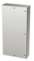
Saginaw Enviroline series enclosure, NEMA 3R/4/4X/12/13, 72 x 36 x 12in (HxWxD), wall mount, 316L stainless steel, #4 brush finish, single-door, 1/4-turn semi-flush latch.
