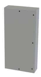
Saginaw Enviroline series enclosure, NEMA 3R/4/12/13, 72 x 36 x 12in (HxWxD), wall mount, carbon steel, ANSI 61 gray, powder coat finish, single-door, 1/4-turn semi-flush latch.
