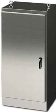
Saginaw Enviroline series enclosure, NEMA 3R/4/4X/12/13, 72 x 30 x 18in (HxWxD), freestanding, 316L stainless steel, #4 brush finish, single-door, 3-point keylocking/padlocking combo handle.
