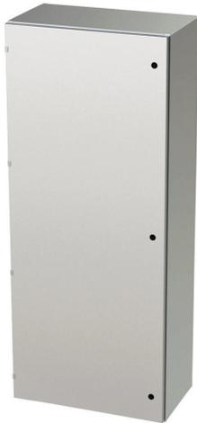
Saginaw Enviroline series enclosure, NEMA 3R/4/4X/12/13, 72 x 30 x 16in (HxWxD), wall mount, 304 stainless steel, #4 brush finish, single-door, 1/4-turn semi-flush latch.
