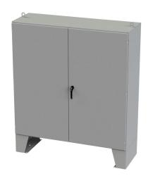
Saginaw enclosure, NEMA 3R/12/13, 72 x 72 x 24in (HxWxD), floor mount, carbon steel, ANSI 61 gray, powder coat finish, double-door, 3-point keylocking/padlocking combo handle.
