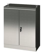
Saginaw enclosure, NEMA 3R/12/13, 72 x 72 x 24in (HxWxD), freestanding, 304 stainless steel, #4 brush finish, double-door, 3-point keylocking/padlocking combo handle.
