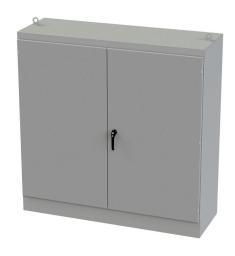
Saginaw enclosure, NEMA 3R/12/13, 72 x 72 x 24in (HxWxD), freestanding, carbon steel, ANSI 61 gray, powder coat finish, double-door, 3-point keylocking/padlocking combo handle.
